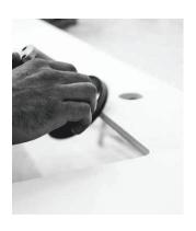
Some stonemasons or Counter top workers work in a traditional way making cuts and holes in the pieces manually. We thus recommend always using wet operation, with suitable tools for porcelain tiles, always in good condition.
